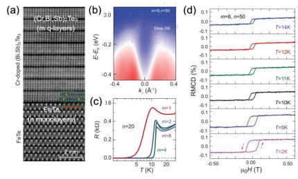
Above (a): HRTEM image of a FeTe/(Cr.Bi.Sb)<sub>2</sub>Te<sub>3</sub> heterostructure. (b) ARPES spectrum of the sample shown in (a). (c) Resistance versus temperature in 3 samples, showing a superconducting transition. (d) RMCD measurements showing the presence of ferromagnetism in a heterostructure even in the superconducting phase.
