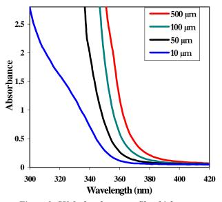
Figure 2. SU-8 absorbance vs. film thickness
