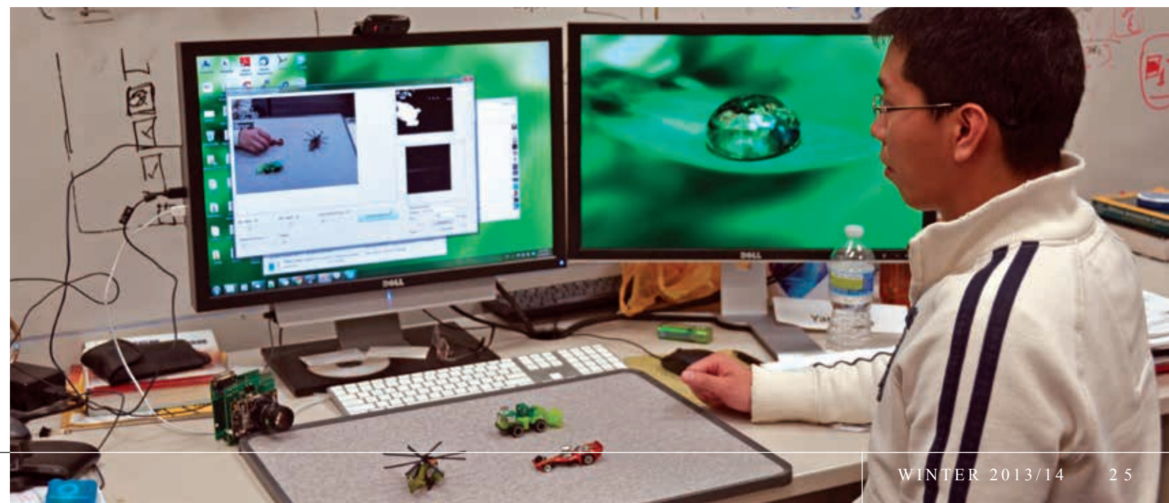
Graduate student Yang Xiao demonstrates a camera that recognizes objects and displays them on a screen, with a bounding box and name of the object.
