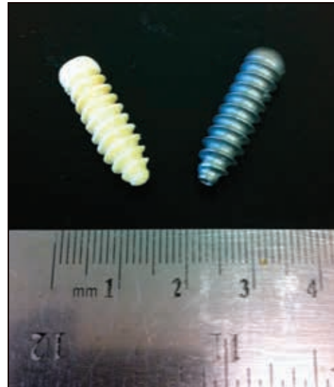
Biodegradable hard polymer bone screws release citric acid to promote healing. Credit: Yang lab
