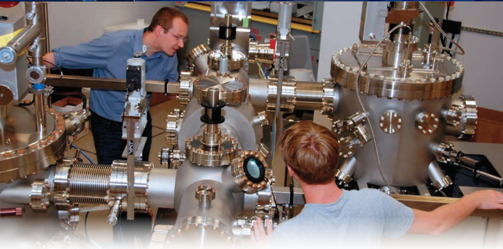
Roman Engel-Herbert with student adjusts the hybrid molecular beam epitaxy instrument in the Millennium Science Complex. Credit: MRI
