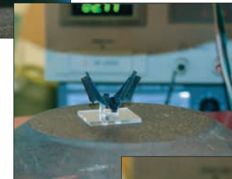
Compliant magnetic materials are activated under an electromagnet in the von Lockette lab to make flapping wings.
