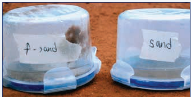
A “stick test” determines if the sand is charged.
