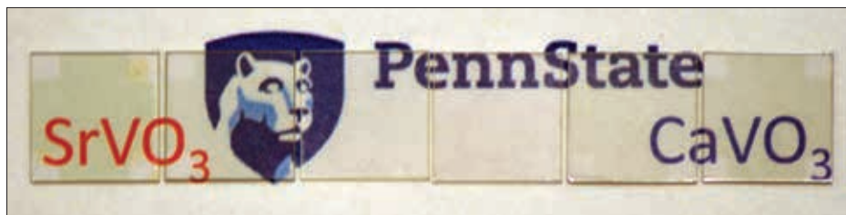
Samples of the correlated metals strontium vanadate (two squares on left) and calcium vanadate (two squares on right) with two uncoated squares in center. The film thickness is 12 nanometers and 4 nanometers on the coated squares. Image credit: MRI/Penn State
