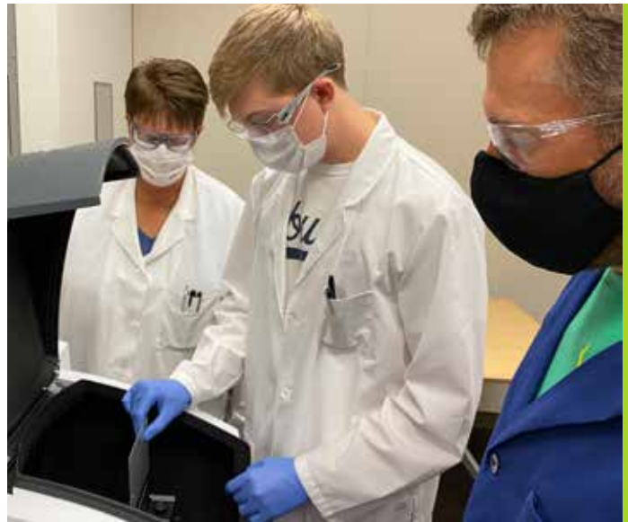
Connor Mosebey (center) loads a materials sample into a UV-Vis spectrometer while Materials Research Institute researchers Nichole Wonderling (left) and Josh Stapleton (right) observe his work in the Millennium Science Complex on the University Park campus. Credit: Penn State MRI
