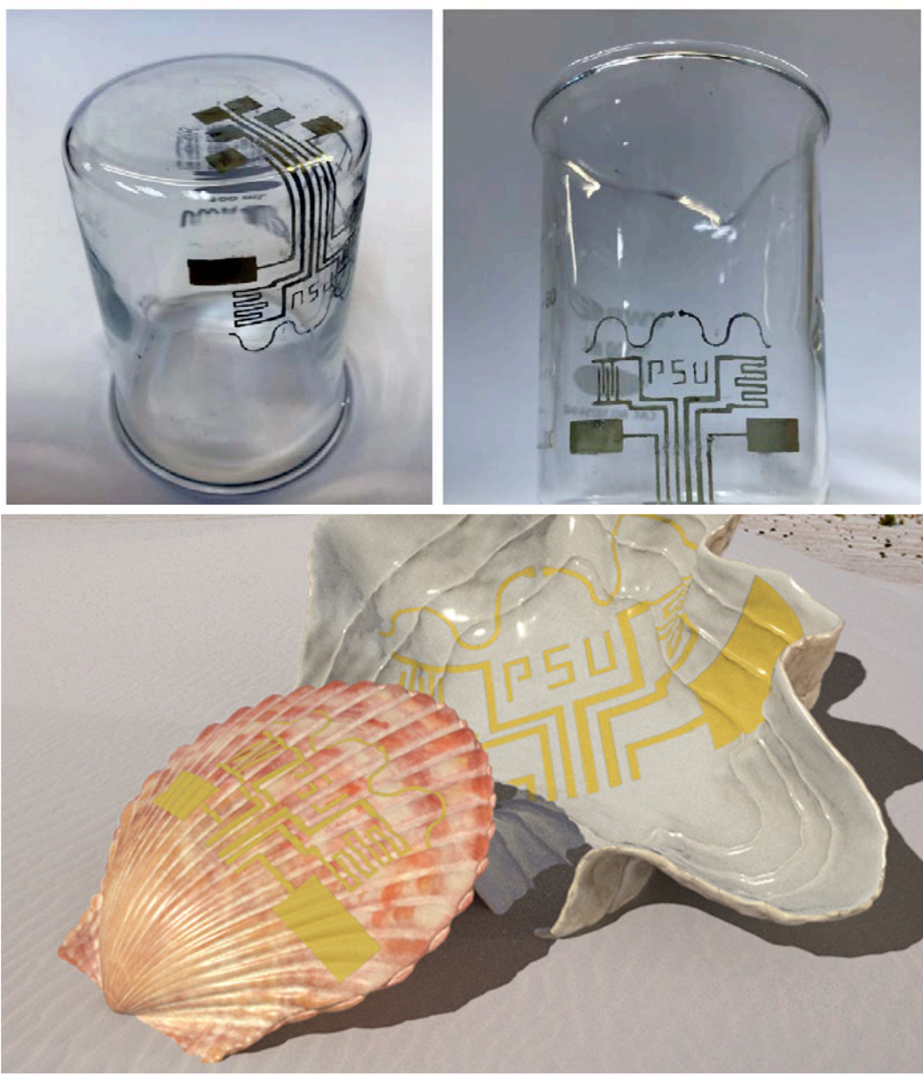
A) and B) Images of a flexible, wearable sensor demonstrated on the curve of beakers. IMAGES: H. Cheng Group C) Sensors show their flexibility to curve on varying textures IMAGE: Jennifer M. McCann/Penn State
