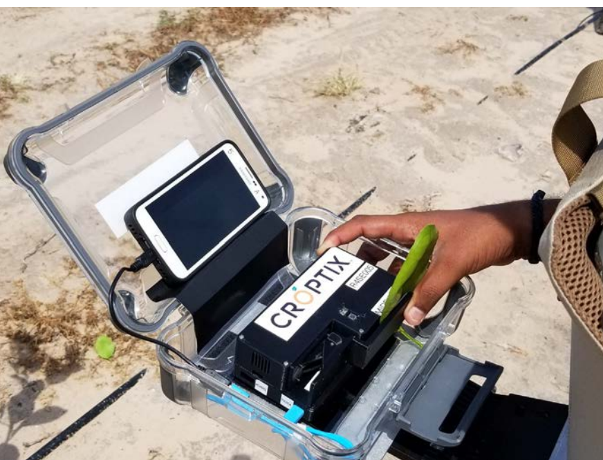
A worker uses the Croptix device to check for Citrus Greening. Image: Croptix
