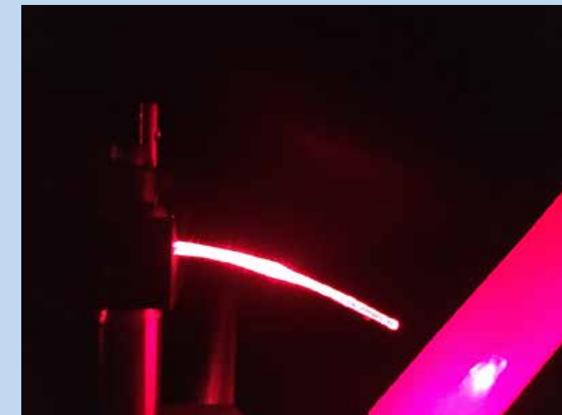
A view of light delivery through a citrate-based optical fiber Credit: D. Shan/C. Zhang / Penn State
