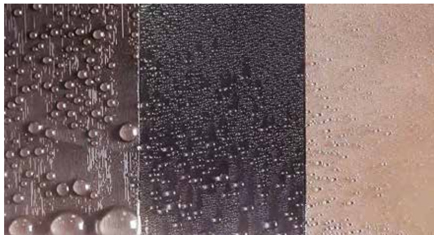
The left panel is a directional slippery rough surface (SRS, this study), the middle panel is a slippery liquid-infused porous surface (SLIPS) and the right panel is a superhydrophobic surface. This image shows a comparison of water harvesting performance of SRS vs other state-of-the-art liquid repellent surfaces.
