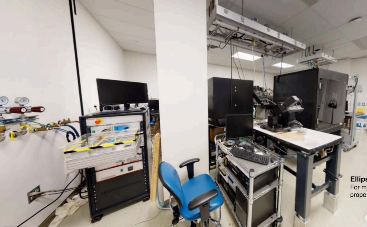
Ellipsometer -For measuring the optical properties and thickness of films.
